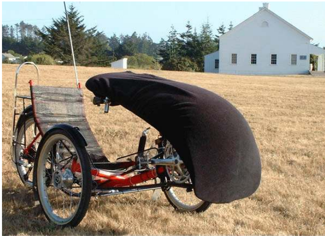
Greenspeed GTO with body sock fairing and AC RSCO cover.
